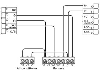
**Note:** Do not jumper Rc or Rh, ecobee3 does this automatically. R can go into either Rc or Rh terminals on your ecobee3.
