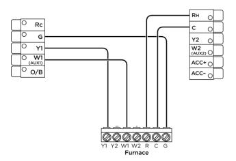
**Note:** Do not jumper Rc or Rh, ecobee3 does this automatically. R can go into either Rc or Rh terminals on your ecobee3.
