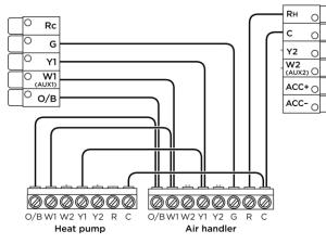
**Note:** Do not jumper Rc or Rh, ecobee3 does this automatically. R can go into either Rc or Rh terminals on your ecobee3.
