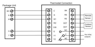
Remote Temperature Sensor Connections and Operation:
