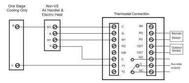
Remote Temperature Sensor Connections and Operation:
