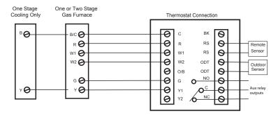
Remote Temperature Sensor Connections and Operation:
