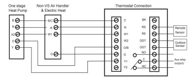
Remote Temperature Sensor Connections and Operation:
